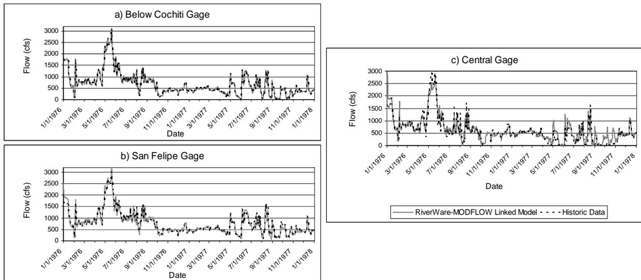
**Figure 4. RiverWare-MODFLOW Linked Model Data as Compared to Historic Flow Data for 3 Gages on the Rio Grande (Below Cochiti, San Felipe and Central). Data is shown for 1976 and 1977.**
