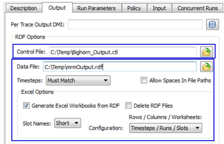
This tab is where the Output is from each run is specified. First, the **RDF Options** (Riverware Data Format) files must be designated. The RDF file is a text file, external to RiverWare, to which all output values are written.
