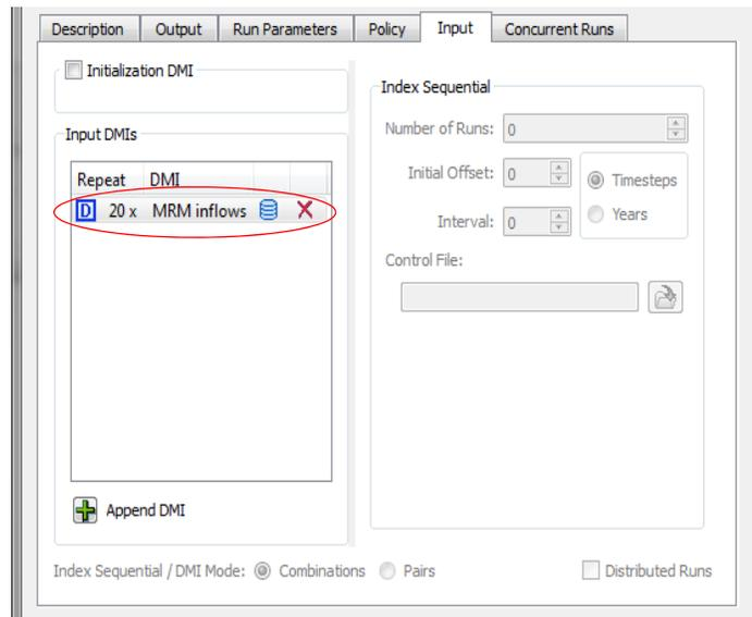
In this tab, we have specified the DMI (**MRM inflows**) to use for the Inputs and how many times to execute it (20x). This means we will run this same DMI before each individual run. Because of the way it is configured, it will know which run it is (run0, run1, ...) and import the correct data. You can further look at the **MRM inflows** DMI from the DMI Manager (**DMI** → **DMI Manager**) and then double click on **MRM inflows**.
