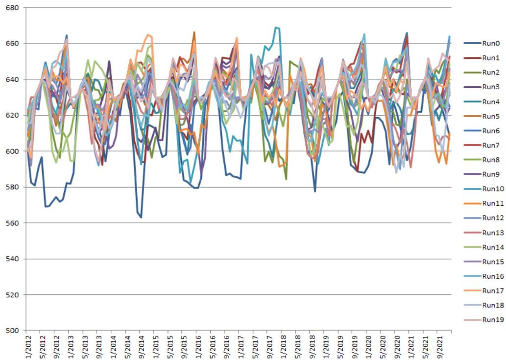
The graph shows the resulting 10 years of pool elevation for each of the 20 hydrologies. This simulation is based on synthesized inputs but it demonstrates the ease of visualizing MRM outputs in Excel.
