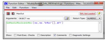
This function computes a number (it's return type is NUMERIC) by evaluating a predefined RiverWare function, **GetMaxOutflowGivenInflow**, at the current timestep when a reservoir, **res** is passed in as an argument.
