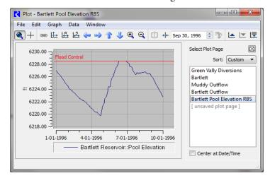
Now that the **BartlettFloodControl** rule is activated, Pool Elevation does not exceed the Flood Control height at any time. Because the rule has the highest priority, no other operation request (i.e. rule) can override it.
